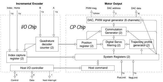
The above figure shows an internal block diagram for the MC1231A motion processor.
