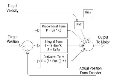
In the PID+Vff filter, the host-specified parameters are:
