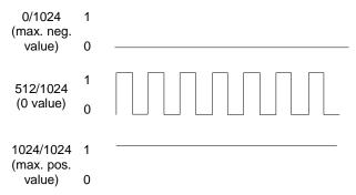
An output pulse width of 0 parts per 1,024 represents the maximum negative voltage, an output pulse width of 512 per 1,024 (50 %) represents a voltage of 0, and a pulse width of 1,024 per 1,024 represents the maximum positive voltage.
