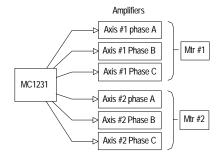
In this configuration the chipset outputs 3 phased PWM magnitude signals per axis. These signals are then fed directly into 3 half-bridge type voltage amplifiers.
